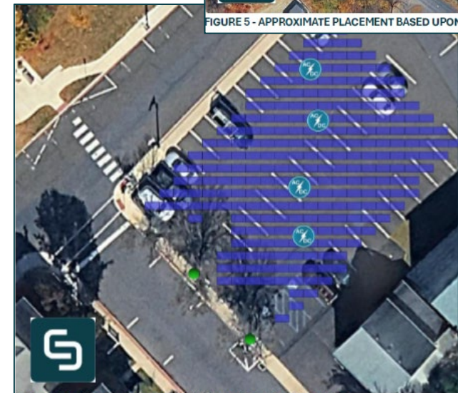
FIGURE 2 - APPROXIMATE PLACEMENT OF SOLAR CANOPIES
